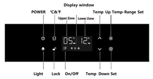
The temperature setting can be adjusted from 5 °C to 20 °C.
