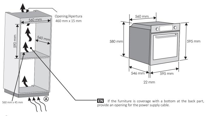
(A) EN If the mounting of the plinth does not allow air circulation, to obtain the maximum performance of the oven it is necessary to create an opening of 500x10mm or the same surface in 5.000 mm<sup>2</sup>
