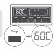
You can gradually decrease the washing water temperature between the maximum temperature and cold washing (--) by pressing washing water temperature adjustment button.
