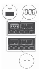
If you have skipped the spinning revolution you want to set, you can re-switch to the revolution by keeping the revolution setting button pressed.
