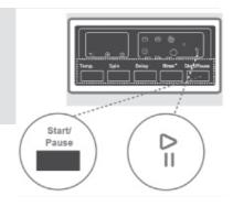
To avoid programme flow from being affected if programme buttons are pressed or programme button is turned when performing washing operation in your machine, child lock is available.
