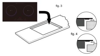
Do not use adhesive to fix the hob into the worktop. Once the seal is fitted position the hob into the cutout in the worktop. Apply gentle downwards pressure onto the hob to push it into the worktop ensuring a good seal around the outer edge (fig. 4)
