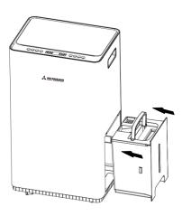
Attention: when the water tank is full of water, please empty it. Before putting the water tank into the dehumidifier, please confirm whether the floater rotates flexibly or not, and then push it in position.
