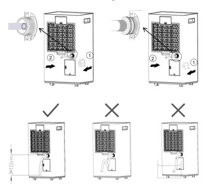
Attention: The external drain pipe must not be too long (recommended length is less than 0.6 meters). The height of the end of the drain pipe must be more than 10cm below the height of the fuselage outlet. The drain pipe must be kept smooth, otherwise the water may not be drained normally.
