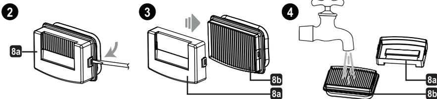
2. Use tool to open the HEPA Filter body 8a .
