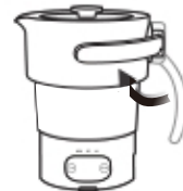
Push the button up, turn the handle to the left, and fold the handle.
