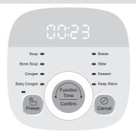
"Function & Time" Knob: Select the function and add/subtract time by rotating the knob. Press the knob to confirm the selection.
