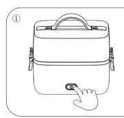
Power on, press the switch button, then the indicator light is on, indicating that the electric lunch box has started.
