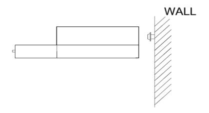
STEP 4 : Tighten the 2 screws completely.
