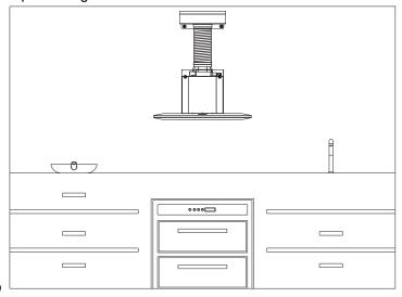
3. Fix the upper chimney to the metal outlet with 2 screws (M4X 10).
