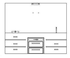
2. Fix the cooker hood and Upper & Bottom chimney in the wall with screws: Secure the sides of the brackets using the 2screws (M4X10) supplied.
